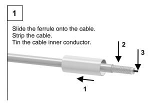
Crimp the ferrule with crimping tool ( see connector TDS ).
